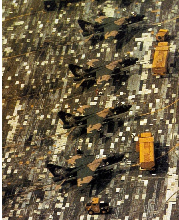
Disruptively camouflaged A-7D Corsairs on a disruptively painted concrete surface, Thailand, 1972 USAF photo
